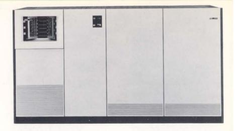
The 2305 is a Fixed Head Storage Facility that provides fast access, high data rate, medium capacity, and modular, direct access storage. This facility consists of a 2835 Storage Control Unit and up to two 2305 Fixed Head Storage Modules.
